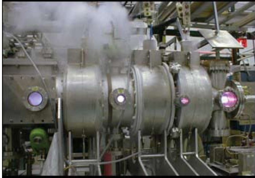
Fig. 1 VASIMR engine under test at NASA-JSC, Houston
