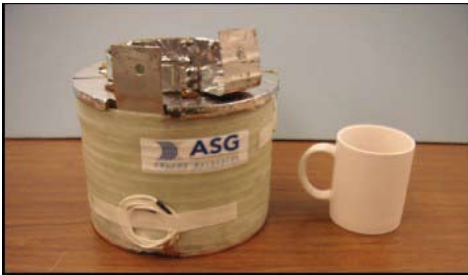
Fig. 2 Superconducting magnet made with MgB2 wire.
